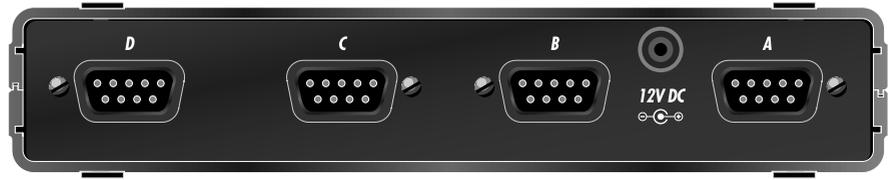
The four ports on the back of the unit connect to the devices being controlled, using the appropriate smartlink cable. Each of the four ports is designated by a letter (A through D) corresponding to the Port pop-up menu in the “Choose Port” dialog box in TRAX (see page 15).
