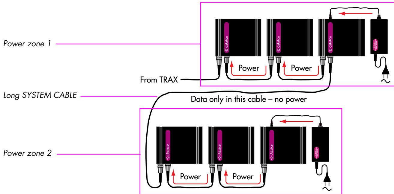
▼ **CAUTION:** Do not attempt to power SMARTPAX QC units that are far apart through the SYSTEM CABLE. Doing so may result in unreliable operation or damage to connected equipment.
