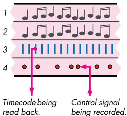
The show can be recorded onto a separate control signal track on tape. This allows you to run the show without using the computer, simply by feeding the control signal into the first unit in the control unit chain. This can be any kind of Datatone control unit equipped with a TAPE or PLAY input on the front panel.
